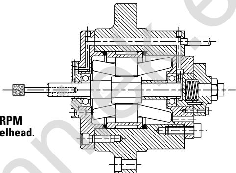
Fig. 113. 100000 RPM high-cycle wheelhead.
