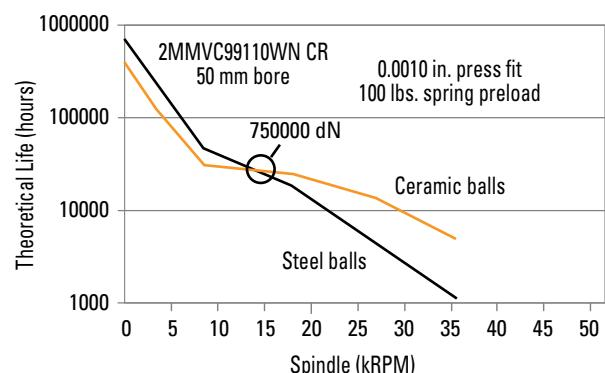
**Fig. 19. L<sub>10</sub> life vs. speed comparison of steel and ceramic balls.**
