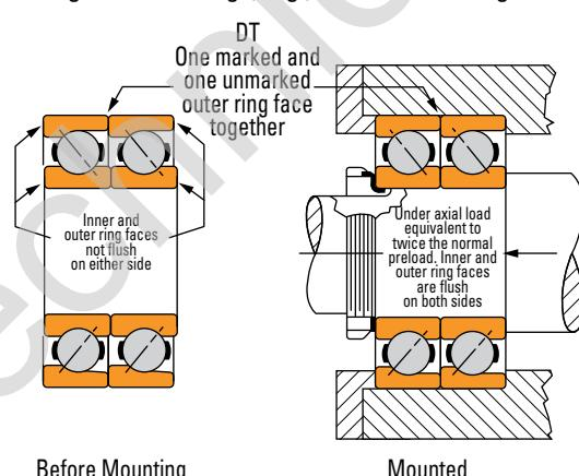
Fig. 85. Tandem bearing assemblies before and after mounting.
