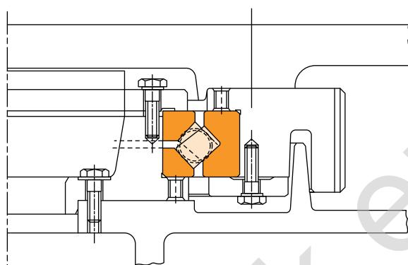
**Fig. 81. Typical mounting arrangement of a TXRDO bearing.**
