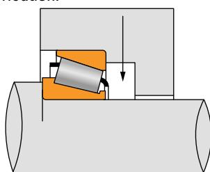
**Fig. 59. Axial oil jet to direct oil at small end of the rollers.**
