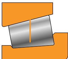
Cone Stand. Cone stand is a measure of the variation in cone raceway size, taper and roller diameter. This is checked by measuring the axial location of the reference surface of a master cup or other type gage with respect to the reference cone face.
