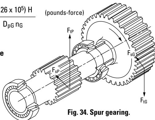
Fig. 34. Spur gearing.
