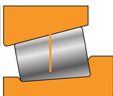
Cup Stand. Cup stand is a measure of the variation in cup I.D. size and taper. This is checked by measuring the axial location of the reference surface of a master plug or other type gage with respect to the reference face of the cup.
