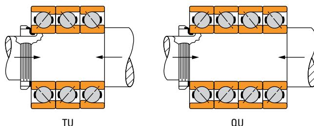
Fig. 86. Typical triplex and quadruplex bearing mountings.
