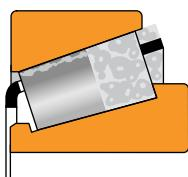
**Fig. 58. Simple radial oil inlet hole with oil collector.**
