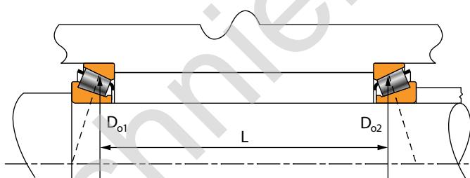
**Fig. 94. Resulting distance between bearing geometric centerlines.**
