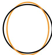
**Runout.** Runout is a measure of rotational accuracy expressed by Total Indicator Reading (T.I.R.). Total displacement is measured by an instrument sensing against a moving surface, or moved with respect to a fixed surface. A radial runout measurement includes both roundness errors and the centering error of the surface that the instrument head senses against.
