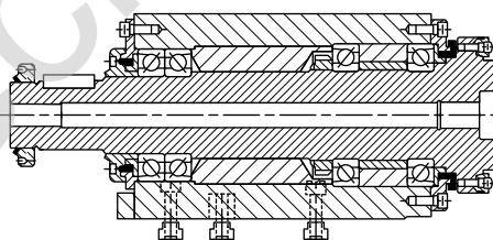
Fig. 107. Heavy-duty precision-boring spindle.
