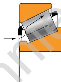
Fig. 55. Pumping effect of a tapered roller bearing
