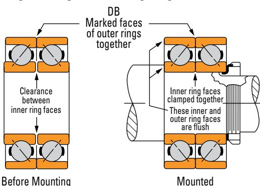
Fig. 83. Back-to-back bearing assemblies before and after mounting.
