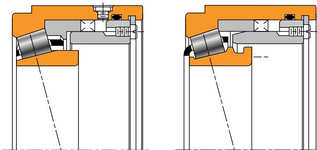
Fig. 78. Two designs of the Hydra-Rib bearing.
