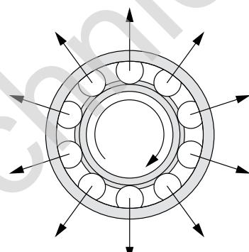
Fig 14. Centrifugal forces of a rotating ball bearing.
