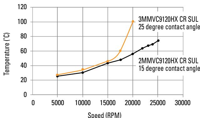
**Fig 16. Effect of contact angle on temperature.**
