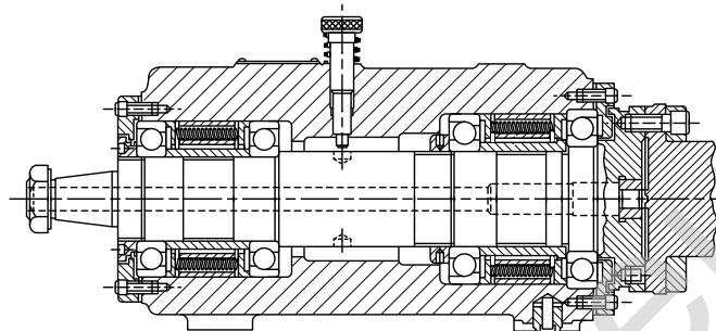
**Fig. 109. High-speed precision-boring head.**
