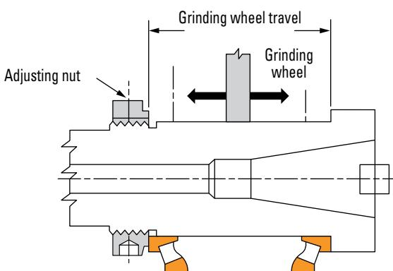
**Fig. 73. Grinding of cone shaft and backing shoulders.**
