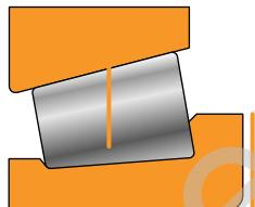
Cone Stand. Cone stand is a measure of the variation in cone raceway size, taper and roller diameter. This is checked by measuring the axial location of the reference surface of a master cup or other type gage with respect to the reference cone face.
