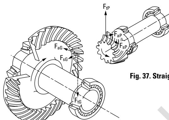
Fig. 37. Straight bevel gearing.
