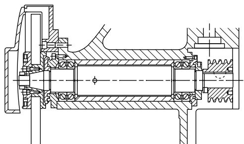
**Fig. 111. Precision toolroom surface grinder spindle.**
