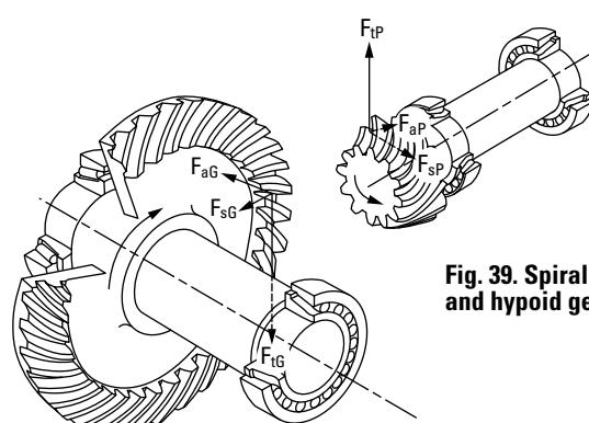
Fig. 39. Spiral bevel and hypoid gearing.
