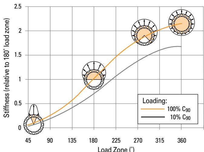
Fig. 5. Effect of load zone on bearing stiffness.
