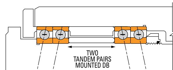
Fig. 91. DT-DB Mounting, fixed (suggested)
