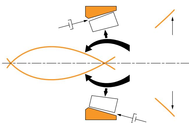
**Fig. 31. Damping in a tapered roller bearing.**
