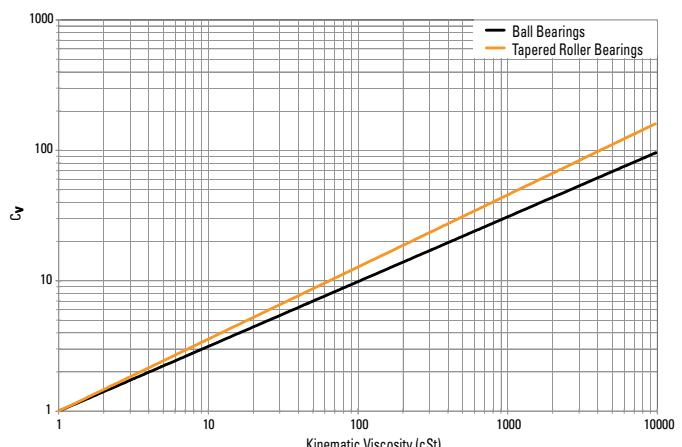
Fig. 52. Viscosity factor ( $C_v$ ) vs. kinematic viscosity.
