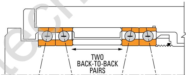
Fig. 89. DB-DB Mounting, fixed (not suggested).
