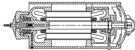
Fig. 116. High-speed motorized router.
