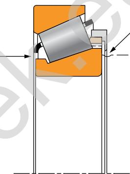
**Fig. 61. The TSMA bearing.**
