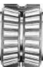
This has a one-piece (double) outer race and two single inner races and is usually supplied complete with an inner ring spacer as a pre-set assembly. This configuration gives a wide effective bearing spread and is frequently chosen for applications where overturning moments are a significant load component. TDO bearings can be used in fixed (locating) positions or allowed to float in the housing bore, for example, to compensate for shaft expansion.
