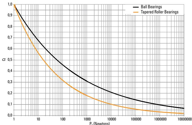
Fig. 48. Load factor ( $C_l$ ) vs. equivalent bearing load ( $P_r$ ).
