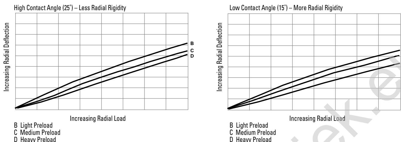
**Fig. 18. Effect of contact angle on radial deflection.**
