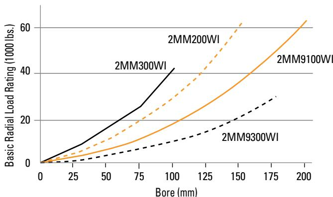
**Fig 20. Angular contact ball bearing load ratings.**
