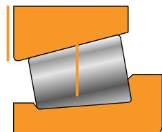
Cup Stand. Cup stand is a measure of the variation in cup I.D. size and taper. This is checked by measuring the axial location of the reference surface of a master plug or other type gage with respect to the reference face of the cup.
