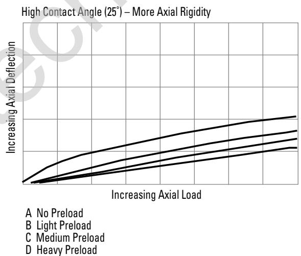
**Fig. 17. Effect of contact angle on axial deflection.**
