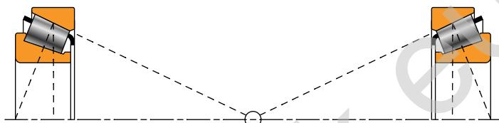
**Fig. 93. Graphical determination of optimum thermal spread.**
