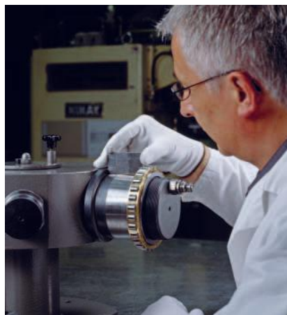
12: Determination of the distance to the shaft shoulder
