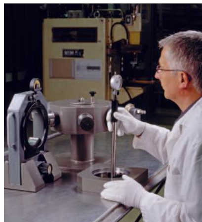
9: Determination of outer ring raceway diameter
