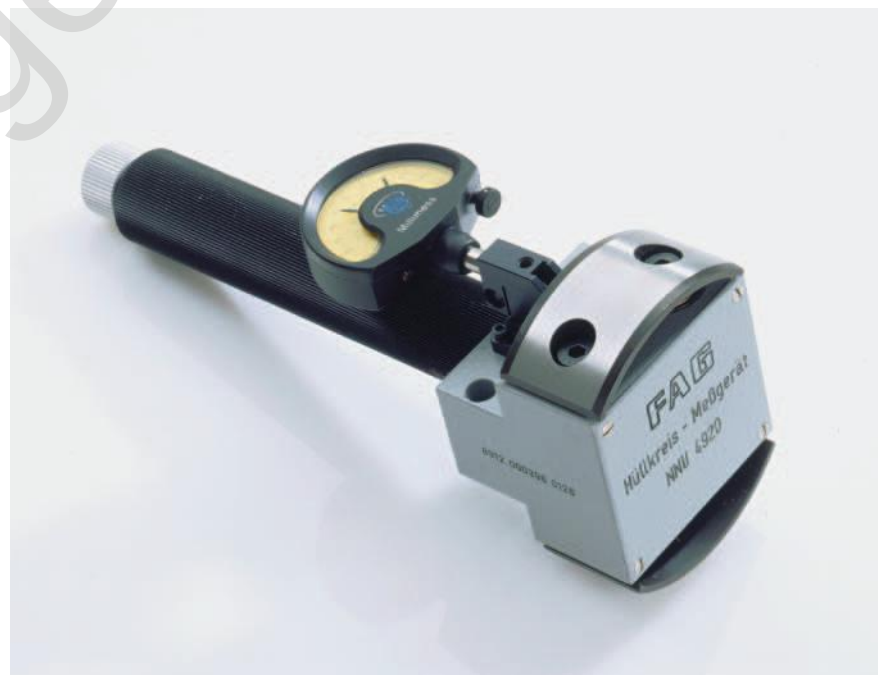
14: FAG enveloping circle gauge MGI 21 for setting the radial internal clearance or preload of cylindrical roller bearings with removable inner ring
